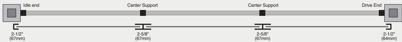
Electroshades using 2-1/2" (64mm) side channels and 2-5/8" (67mm) center channels.
